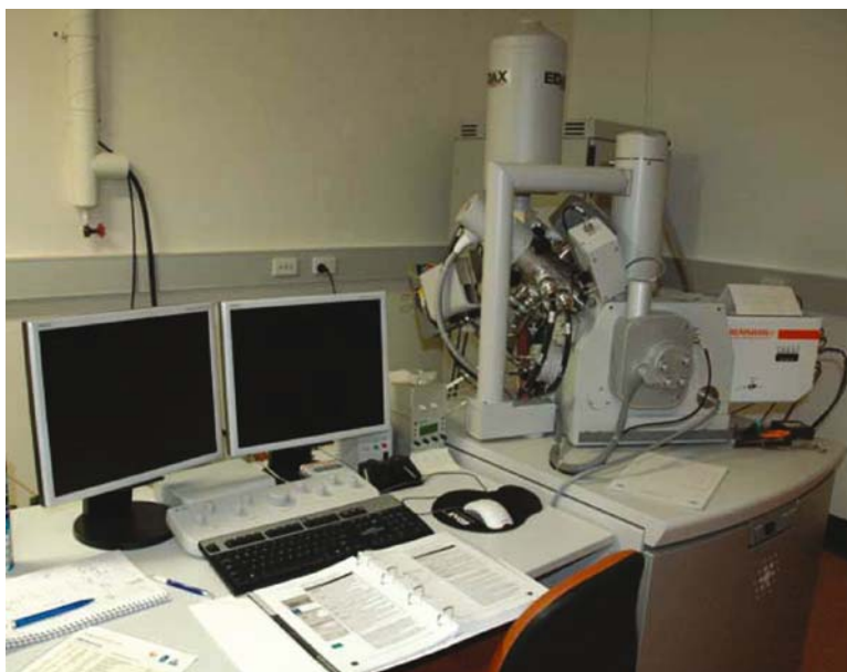
Fig. 15.12. FEI QUANTA 200 3D integrated equipment platform. This dual SEM/FIB workstation is currently installed at the University of Sydney
