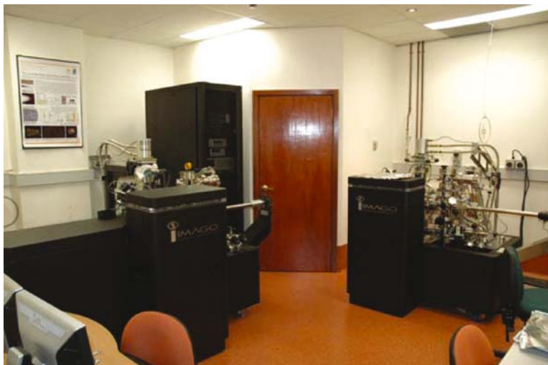
Fig. 15.8. The two LEAP 3000X installed in the AMMRF national atom probe laboratory at the University of Sydney
