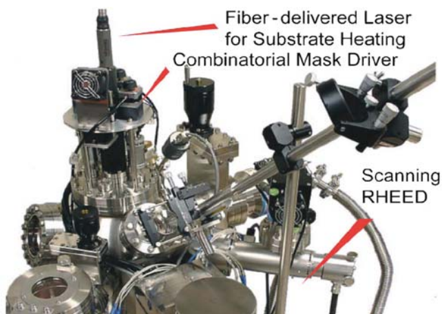
Fig. 4.3. A picture of a compact pulsed laser deposition system equipped with all the capabilities shown in Fig. 4.2 [27]
